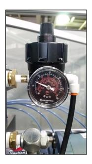
Set the air cylinder pressure between 10 and 15 psi. (Avg. is 14 psi.)
