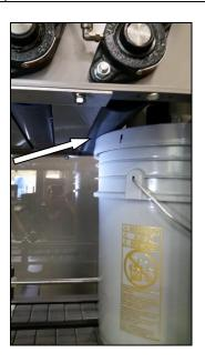
Turn the crank handle to adjust the Entry Roller height adjuster screw.
