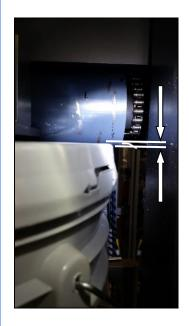
Turn the crank handle to set the exit roller height adjuster screw.
