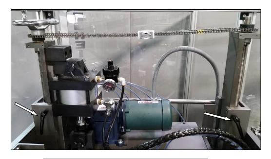
Loosen both lock handles on adjuster slides.
