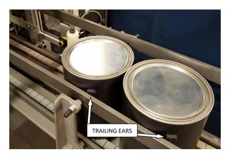
With the conveyor running in automatic mode, flag the photo eye to release the cans. The can leaving the escapement should not get closer than 5/8" to 3/4" from the can receiving the bail.
