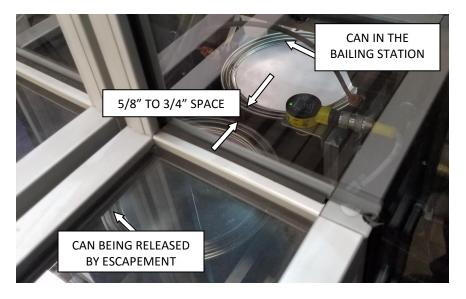
Adjust the escapement photo eye bracket downstream for more space, and upstream for less space.
